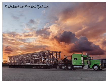
FIGURE 2. The components in truckable process modules, including columns, vessels and tanks, should remain within a 12-by-14 foot footprint in order to fit on the truck for transportation to the site. Shown here is a process module designed and built by Koch Modular Process Systems
