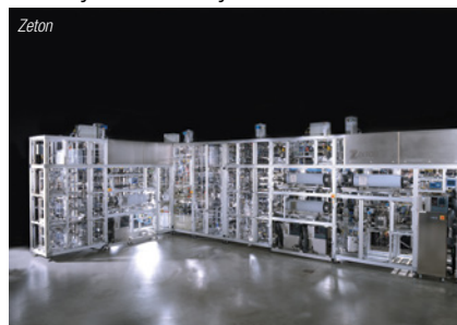
FIGURE 5. For applications that have a high-value/low-volume output, such as designed drugs and semi-conductor chemicals, going modular addresses the need for cost effectiveness and when done via a pre-validated, standardized process module, such as Zeton's ContiUnity technology, it allows a continuous process
